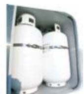
Dual LPG Tanks with Auto Change-over Regulator
