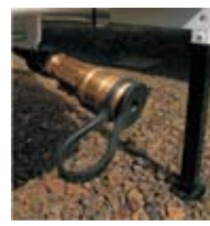
Quick Connect LPG Hook- up For Barbeque and other Exterior Appliances
