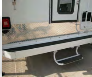
Diamond Plate Kick Panels. Storage in Bumper w/ Locking Doors at Both Ends.
