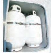
Dual 30 LPG Tanks w/Auto Change-over Regulator
