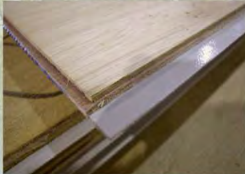
Multi Layered Laminated Fiberglass Wall
