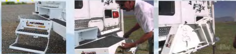
1. Steps in the down position. 2. Treads fold up.... 3. Landing folds up, and pin locks it into place
