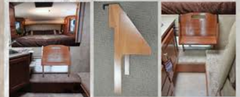
3. Landing folds up, and pin locks it into place
