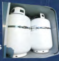
Dual LPG Tanks Dual 30# LPG Tanks w/Auto Change-over Regulator and Lock-able Security Strap
